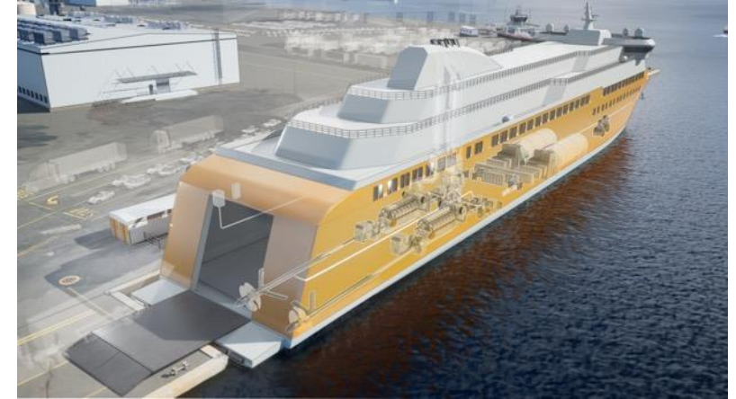
Hybrid propulsion (400 MWh batteries)
