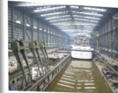
AIDA Nova was floated out at Meyer Werft in May and is due to become the first cruise ship using LNG for propulsion upon its delivery in November.
